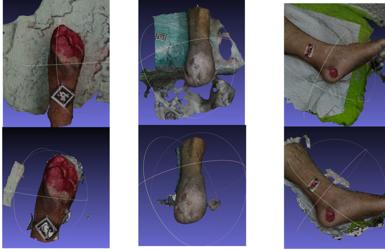
Figure 6.3: Example of 3 cases where the background removal treatment was applied. Baseline 3D models with reconstructed background objects (top) and corresponding 3D models once the background removal process is implemented (bottom).
