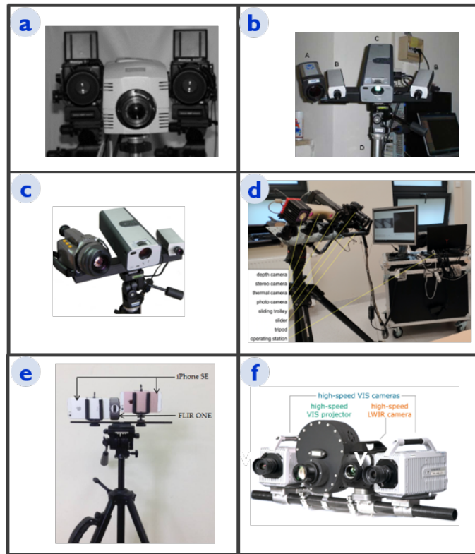
Figure 5.6: Stationary thermal 3D model systems. Images obtained from [101] (a), [30] (b), [12] (c), [51] (d), and [105] (e), [53] (f).
